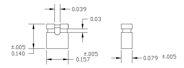
MATERIAL: HOUSING: 30± GLASS FILLED PBT (UL 94V-0) BLACK
