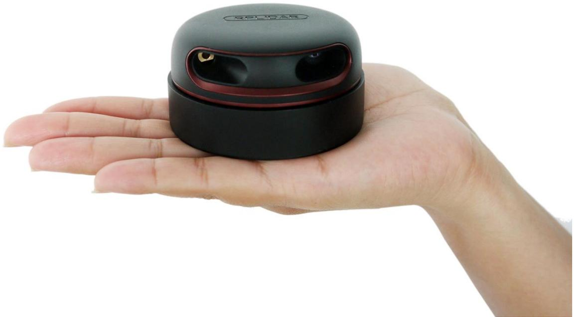
The RPLIDAR A2 is the next generation low cost 360 degree 2D laser scanner (LIDAR) solution developed by SLAMTEC. It can take up to 4000 samples of laser ranging per second with high rotation speed. And equipped with SLAMTEC patented OPTMAG technology, it breakouts the life limitation of traditional LIDAR system so as to work stably for a long time.
