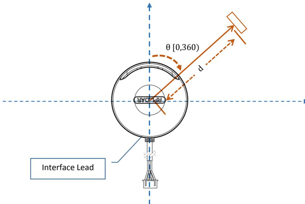
*Figure 2-5 RPLIDAR Scanning Data Coordinate System Definition*
