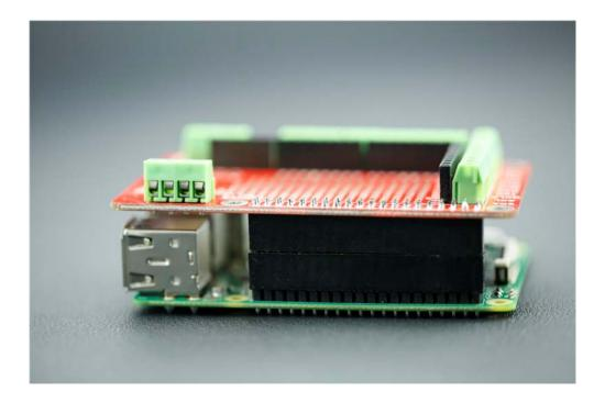
Note: Raspberry Pi and Shield can't be powered simultaneously.
