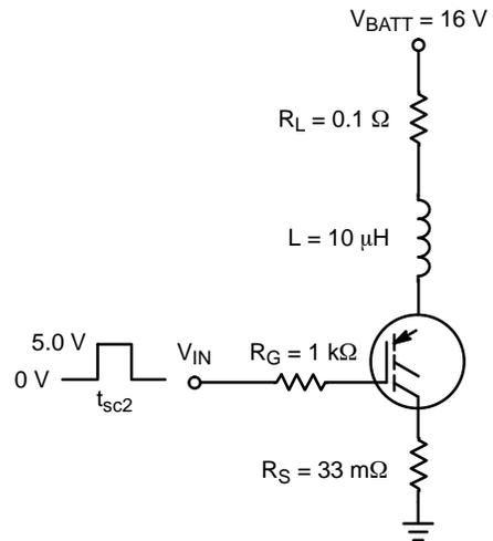
**Figure 18. Circuit Configuration for Short Circuit Test #2**
