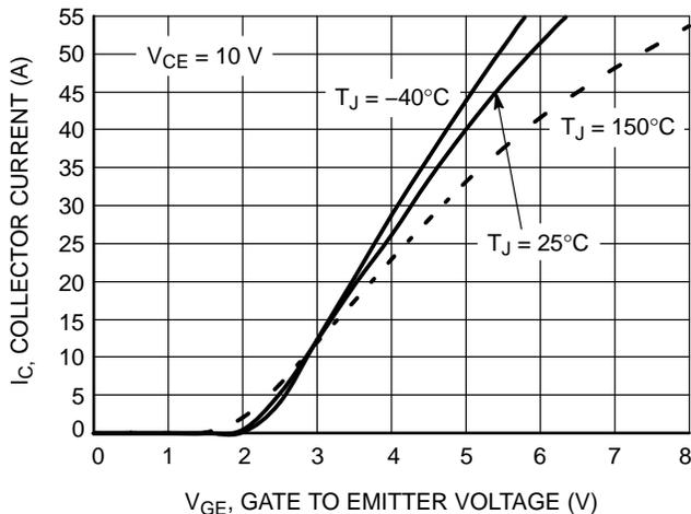
Figure 4. Transfer Characteristics
