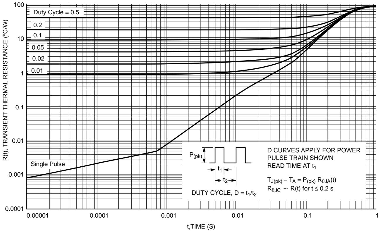
**Figure 19. Transient Thermal Resistance
