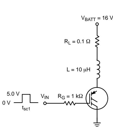
**Figure 17. Circuit Configuration for Short Circuit Test #1**
