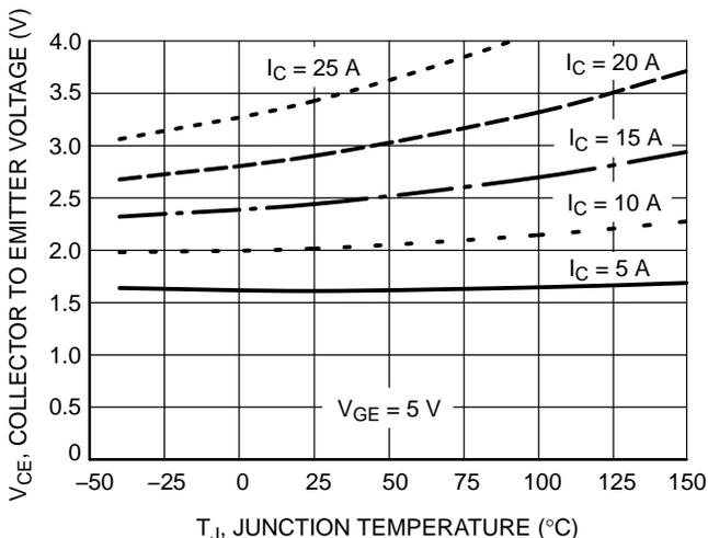
Figure 5. Collector-to-Emitter Saturation Voltage vs. Junction Temperature
