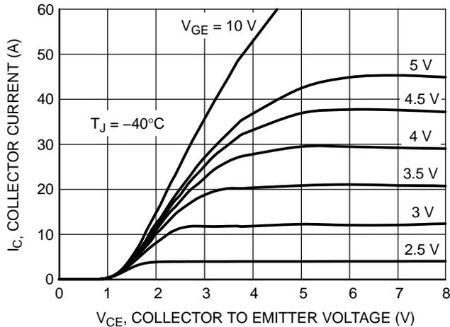
Figure 2. Output Characteristics
