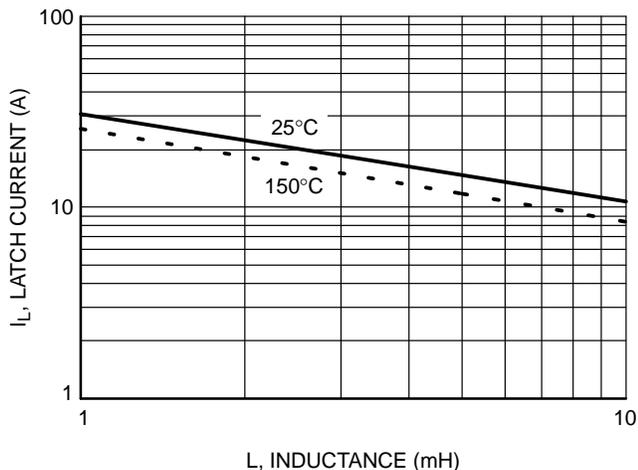
**Figure 11. Typical Open Secondary Latch Current vs. Inductance**
