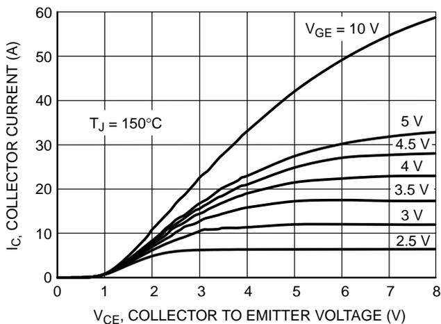
Figure 3. Output Characteristics
