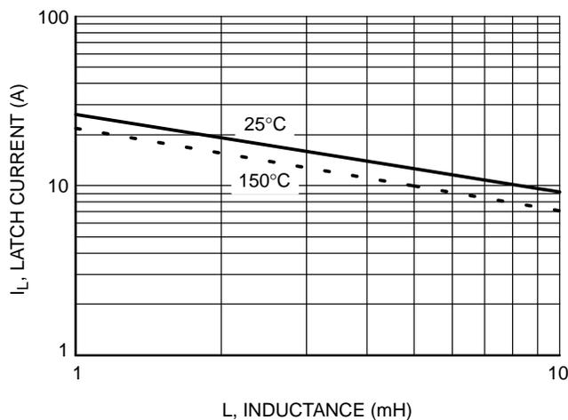
**Figure 10. Minimum Open Secondary Latch Current vs. Inductance**
