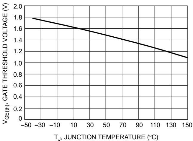
**Figure 9. Gate Threshold Voltage vs. Junction Temperature**
