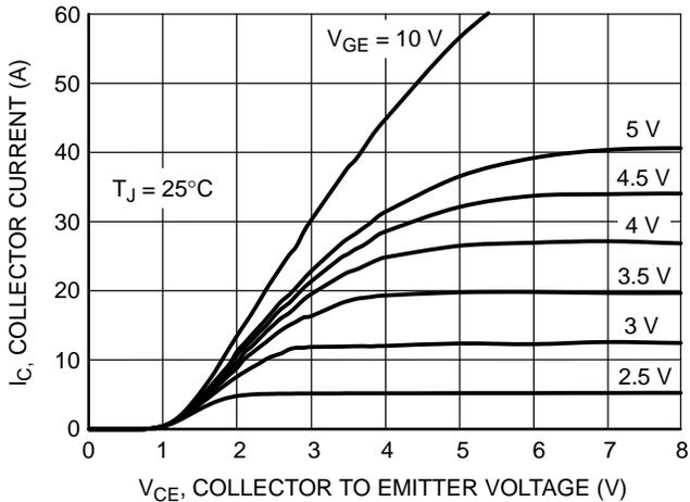
Figure 1. Output Characteristics
