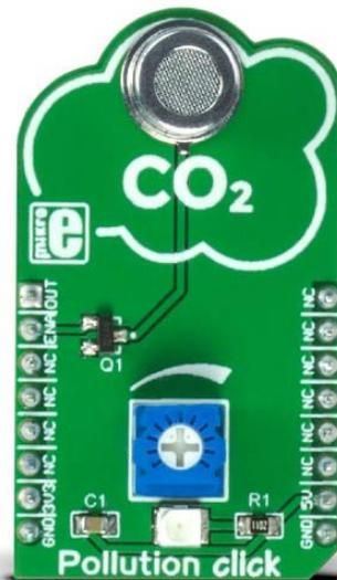
**Pollution click** has high sensitivity to organic gases such as methanal (also known as formaldehyde), benzene, alcohol, toluene, etc. The click carries the WSP2110 VOC gas sensor with the detection range of 1 ~ 50ppm (parts per million).
