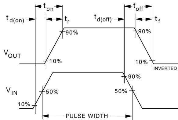
**Figure 12. Switching Waveforms.**
