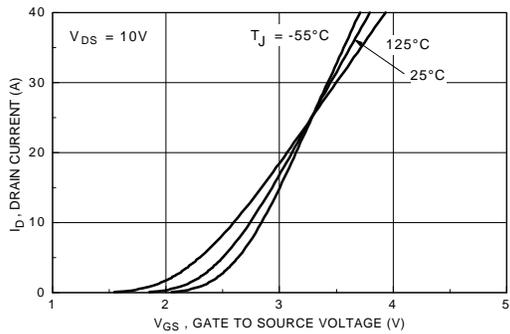
Figure 5. Transfer Characteristics.
