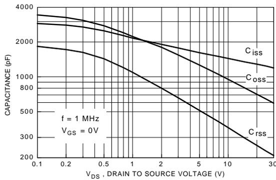
**Figure 9. Capacitance Characteristics.**
