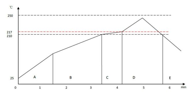
Zone A: Preheat: This raises the temperature at a controlled rate, typically 0.5 - 2C/s. This will preheat the component to 120°C to 150°C to distribute the heat uniformly to the PCB.
