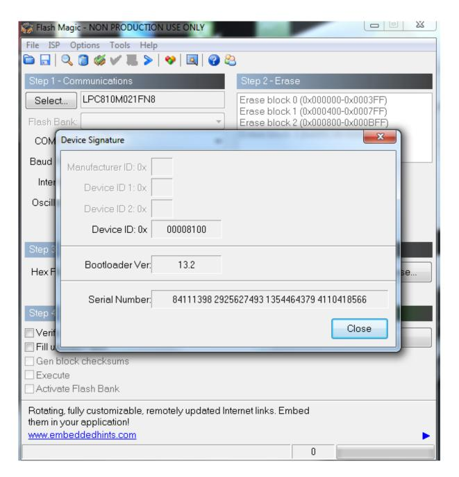
If you get an error message, check your COM port and the connections to your USB to TTL cable and ensure that the ISP pin is pulled low to GND before powering or resetting your board.
