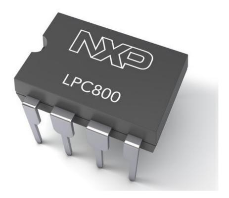
The LPC810 is a new microcontroller from NXP, a super fast little controller has only 8 pins but packs a lot of punch with a high speed processor and 32 bit instructions. This learning guide will show you everything you need to know to get started with the ARM Cortex M0+ based LPC810 microcontroller. It will cover:
