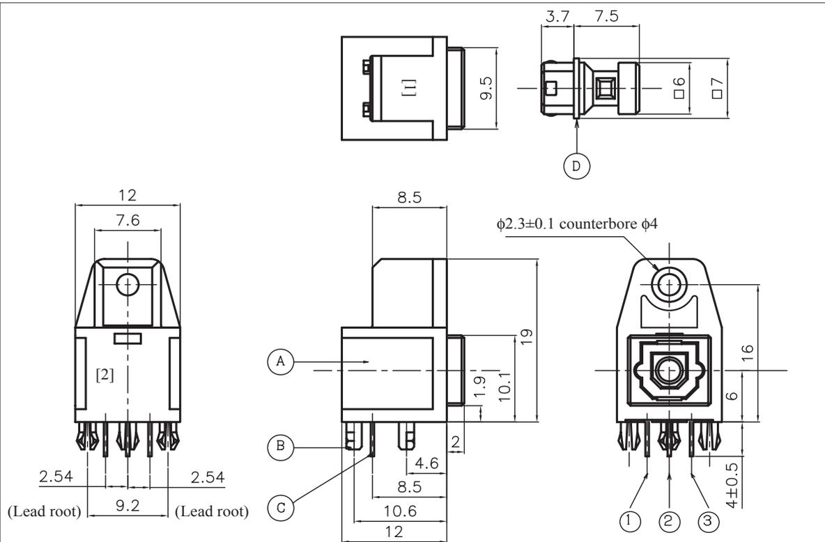
Example of mounting drawing from solder side.
