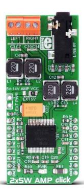
**2x5W AMP click** functions as an amplifier and features the TDA7491LP 2x5-watt dual BTL class-D audio amplifier. The click is designed to run on either 3.3V or 5V power supply. It communicates with the target MCU over the following pins on the mikroBUS<sup>TM</sup> line: AN, RST, CS, PWM, INT.
