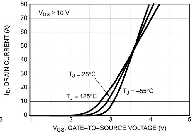
Figure 2. Transfer Characteristics
