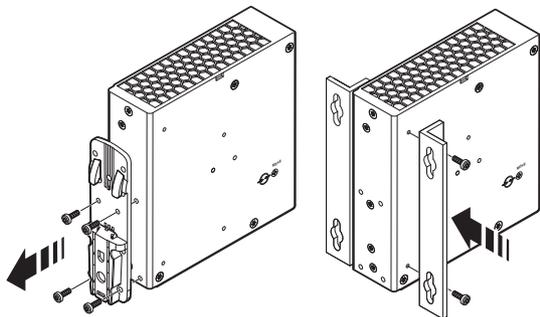
Figure 12 Mounting the UWA 130 universal wall adapter
