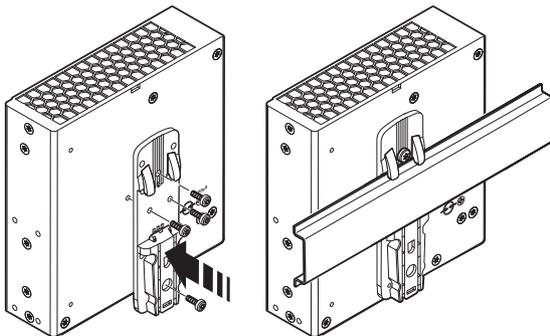
Figure 10 Mounting the universal DIN rail adapter
