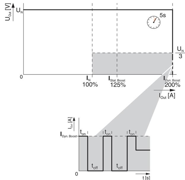
Figure 16 U/I Advanced output characteristic curve
