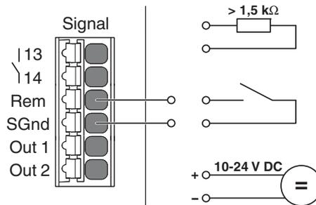
Figure 25 External wiring versions, disable SLEEP MODE
