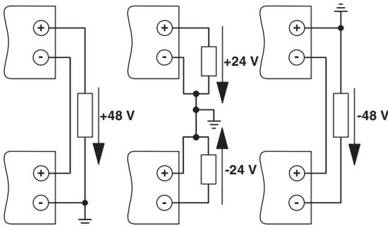
Figure 29 Schematic diagrams in series operation
