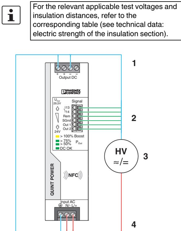
Figure 1 Potential-related wiring for the high-voltage test
