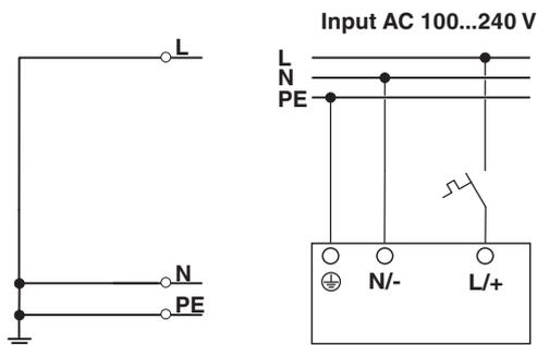
Figure 14 Pin assignment for AC supply voltage
