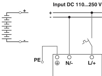
Figure 15 Pin assignment for DC supply voltage
