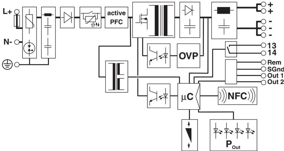
Figure 6 Block diagram
