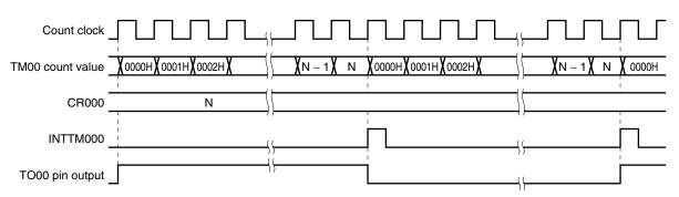
Figure 6-28. Square-Wave Output Operation Timing
