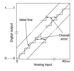
Figure 10-14. Quantization Error
