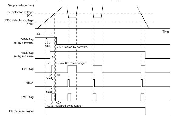
Figure 16-5. Timing of Low-Voltage Detector Interrupt Signal Generation
