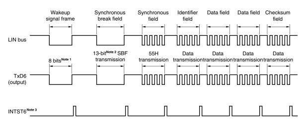
Figure 11-1. LIN Transmission Operation
