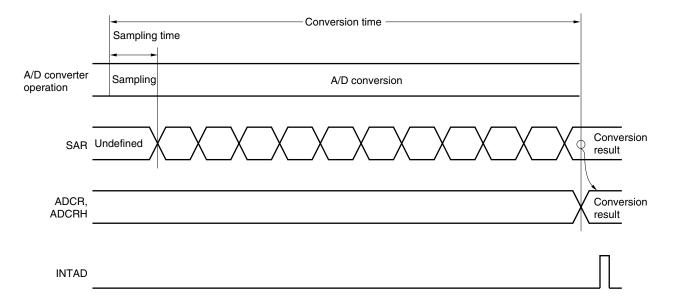
Figure 10-10. Basic Operation of A/D Converter
