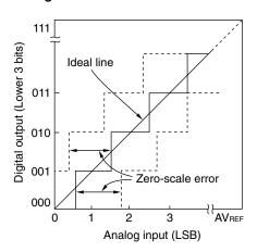
Figure 10-17. Integral Linearity Error
