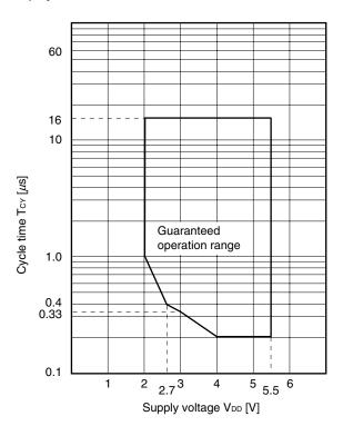
Tcy vs. VdD (High-Speed Internal Oscillation Clock)
