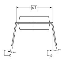
(UNIT:mm) ITEM DIMENSIONS 17.57 MAX. D 6.60 Ε 3.70 MAX. Α 0.65±0.10 Α1 A2 2.80 1.778 е e1 7.62  $0.52 \pm 0.10$ b b1 1.02±0.10 0.77±0.10 b2 С 0.27±0.07 2.86±0.20 0.25  $\theta$  $0^{\circ}$  to  $5^{\circ}$ Ζ 0.609 P20CS-70-CAC
