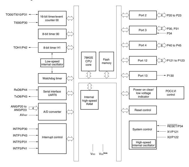
**Note** In the 78K0S/KA1+, Vss functions alternately as the ground potential of the A/D converter. Be sure to connect Vss to a stabilized GND (= 0 V).
