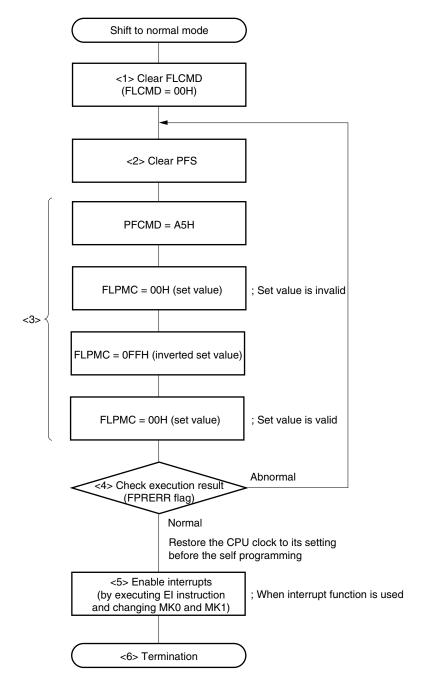
Figure 18-19. Example of Shifting to Normal Mode
