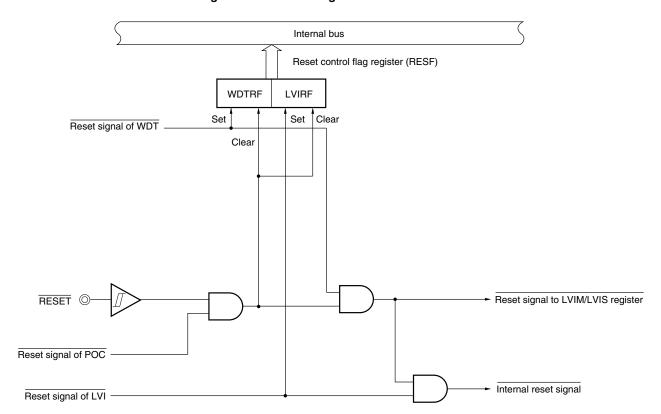
Figure 14-1. Block Diagram of Reset Function
