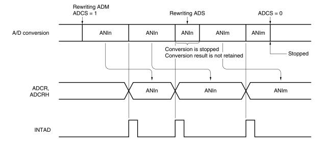
Figure 10-12. A/D Conversion Operation
