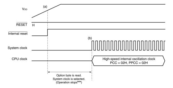
Figure 5-8. Timing Chart of Default Start by High-Speed Internal Oscillation
