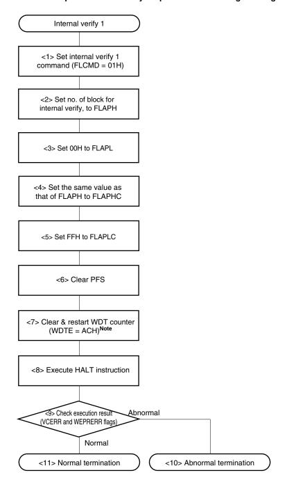
Figure 18-23. Example of Internal Verify 1 Operation in Self Programming Mode
