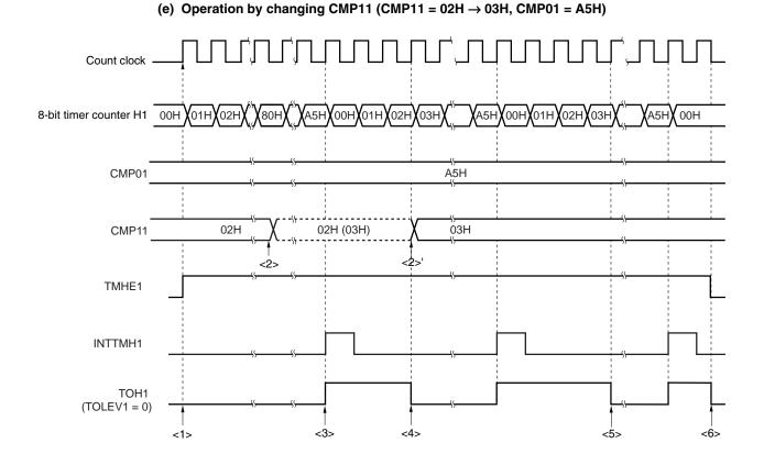
Figure 8-9. Operation Timing in PWM Output Mode (4/4)
