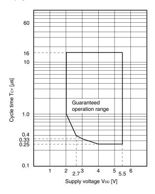
Tcy vs. VDD (High-Speed Internal Oscillation Clock)
