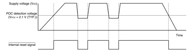
Figure 15-2. Timing of Internal Reset Signal Generation in Power-on-Clear Circuit
