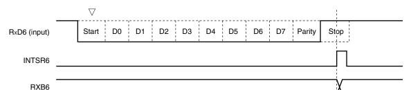
Figure 11-19. Reception Completion Interrupt Request Timing
