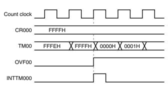
Figure 6-37. Operation Timing of OVF00 Flag
