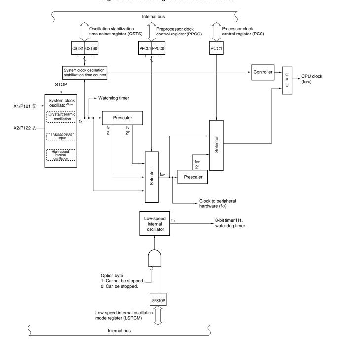
Figure 5-1. Block Diagram of Clock Generators
