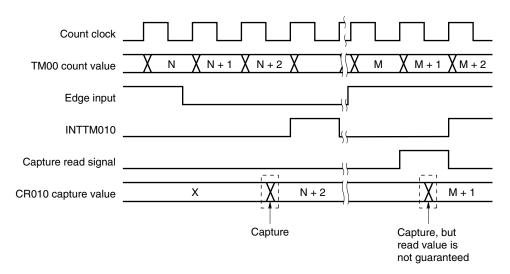
Figure 6-38. Capture Register Data Retention Timing
