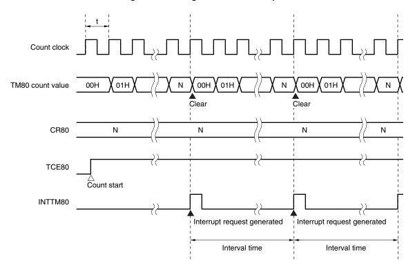
Figure 7-5. Timing of Interval Timer Operation
