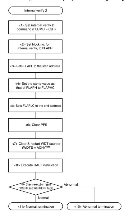
Figure 18-24. Example of Internal Verify 2 Operation in Self Programming Mode
