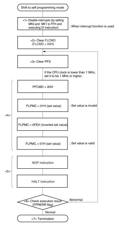
Figure 18-18. Example of Shifting to Self Programming Mode
