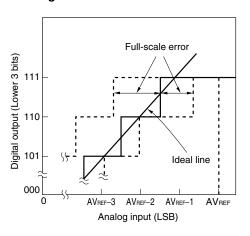
Figure 10-18. Differential Linearity Error
