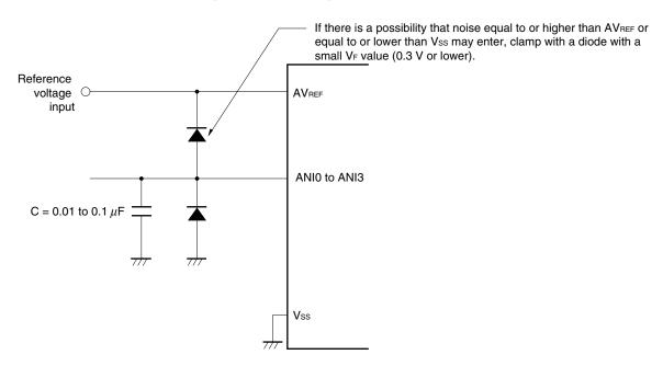
Figure 10-19. Analog Input Pin Connection
