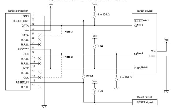
Figure 19-1. Recommended Circuit Connection
