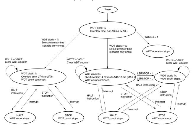
Figure 9-5. Status Transition Diagram When "Low-Speed Internal Oscillator Can Be Stopped by Software" Is Selected by Option Byte
