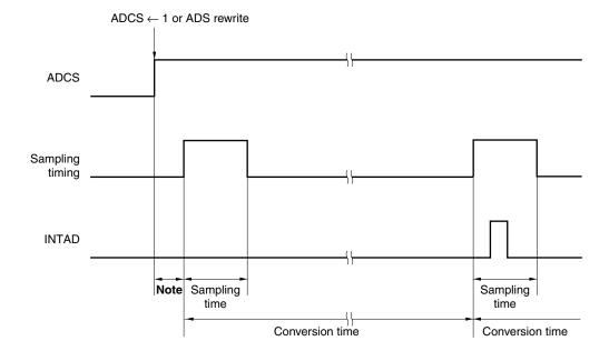
Figure 10-1. Timing of A/D Converter Sampling and A/D Conversion
