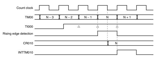
Figure 6-17. CR010 Capture Operation with Rising Edge Specified
