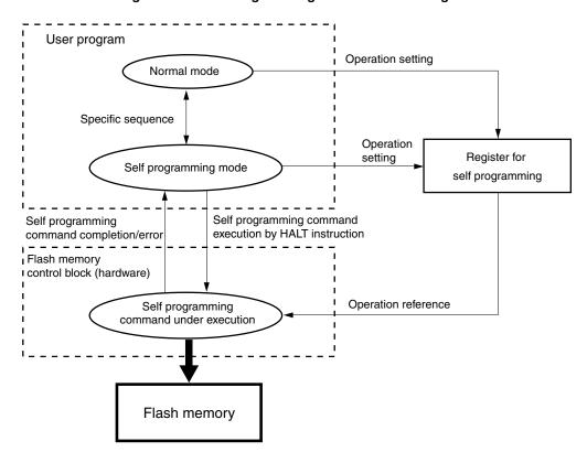
Figure 18-9. Self Programming State Transition Diagram
