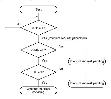
Figure 12-7. Interrupt Request Acknowledgment Processing Algorithm
