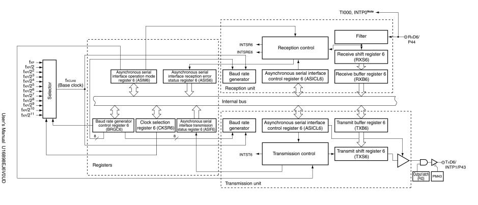
Figure 11-4. Block Diagram of Serial Interface UART6
