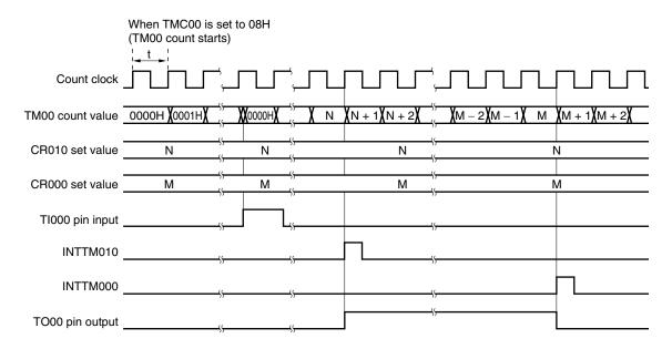
Caution 16-bit timer counter 00 starts operating as soon as a value other than 00 (operation stop mode) is set to the TMC002 and TMC003 bits.
