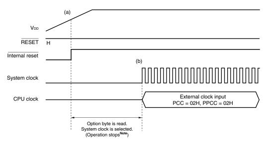
Figure 5-12. Timing of Default Start by External Clock Input
