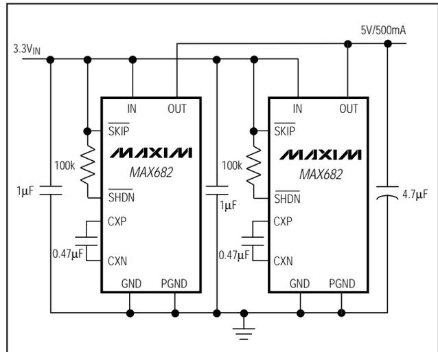
Figure 6. Paralleling Two MAX682s
