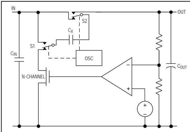
Figure 4. Constant-Frequency-Mode Regulation
