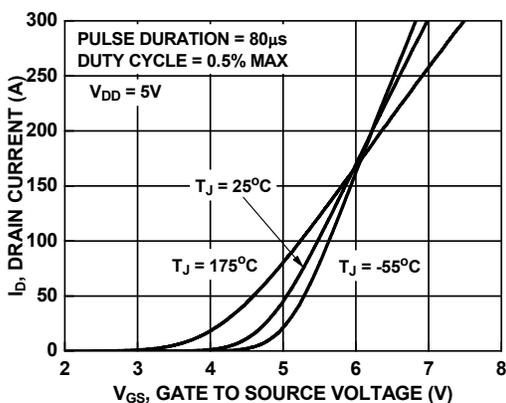
Figure 7. Transfer Characteristics
