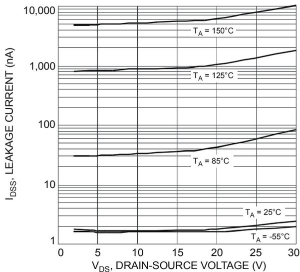
Fig. 11 Typical Leakage Current vs. Drain-Source Voltage
