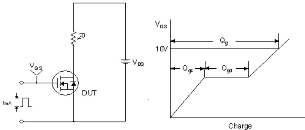
**Resistive Switching Test Circuit & Waveforms**
